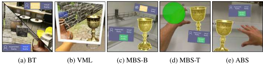
Figure 6.2: To enable transition of objects between VE and AE we created the following five techniques: (a) Binary Transition (BT) , (b) Virtual Magic Lens (VML) , two version of Manual Blended Space : (c) Manual Blended Space - Button transition (MBS-B) and (d) Manual Blended Space - Touch transition (MBS-T) , and (e) Auto Blended Space (ABS) .
